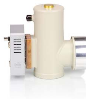
Figure 2-1 : Side view of cougar camera with grey electronics box (left) and vacuum dewar (right)
