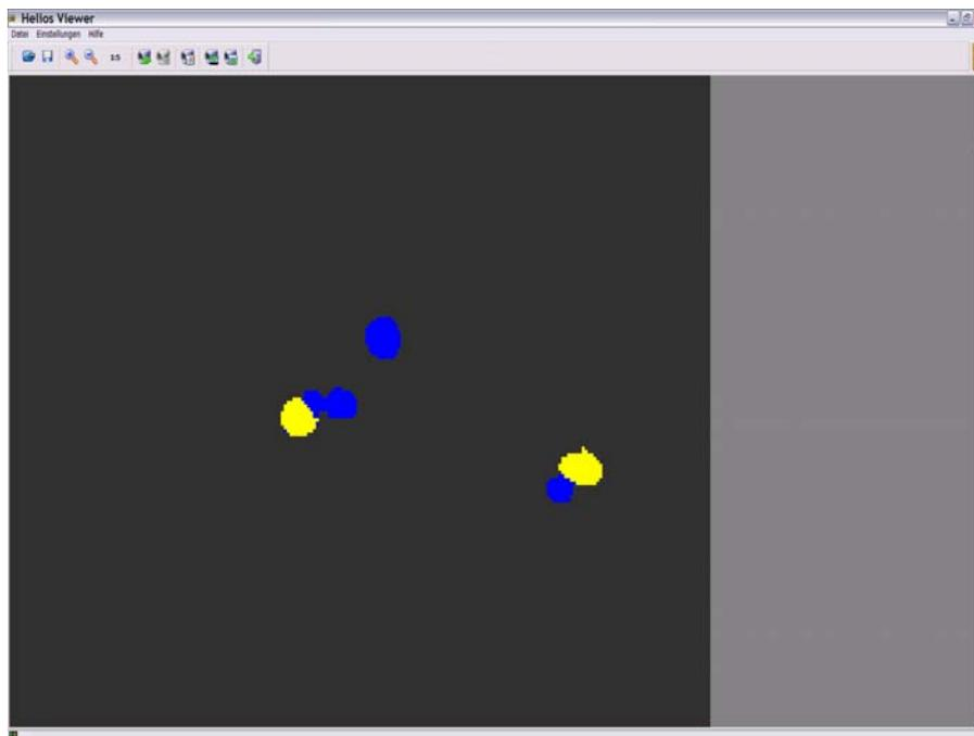
Fig. 4: Live recording of blueberries and blueberry leaves. The classified data acquired by **HELIOS Class** are shown (blueberries in yellow and blueberry leaves in blue). For the objects to be ejected (blueberry leaves), **HELIOS Complete** would additionally fade in the control signal for the ejector in the right part of the image.
