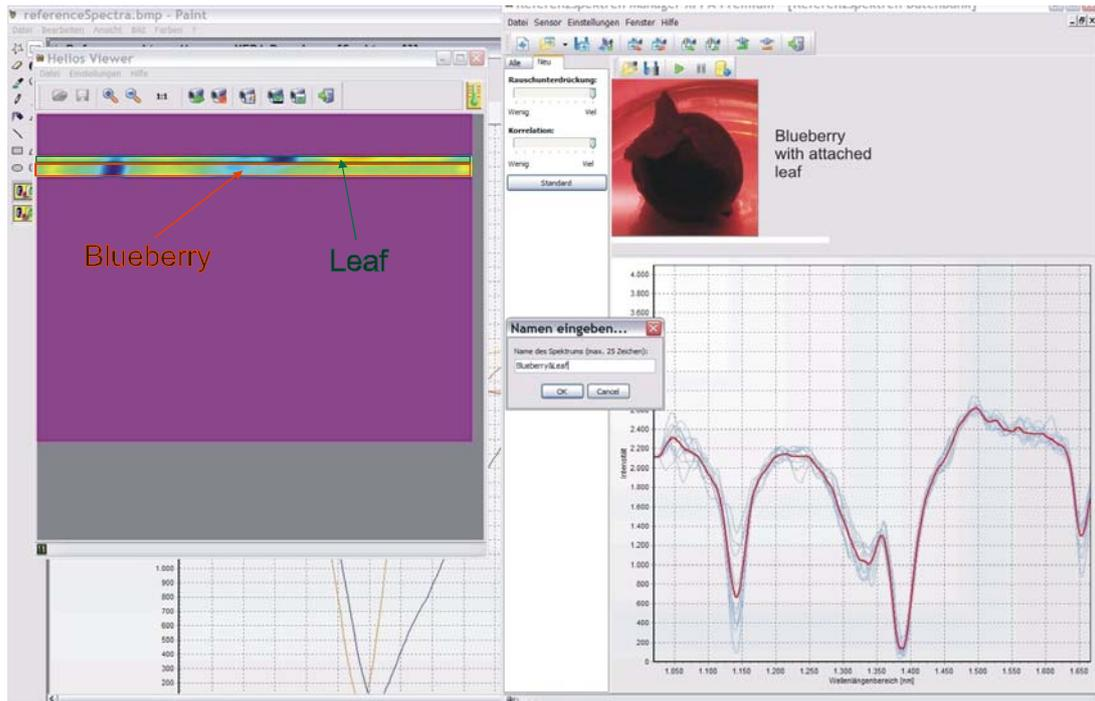
Fig. 6: Recording of a blueberry to which a leaf, whose colour does not differ from that of the blueberry, adheres. In the left part of the image, the different spectra of the leaf (top) and blueberry (bottom) can be identified clearly. As described above, “top” and “bottom” go hand in hand with different local coordinates on the test object “Blueberry with leaf”.
