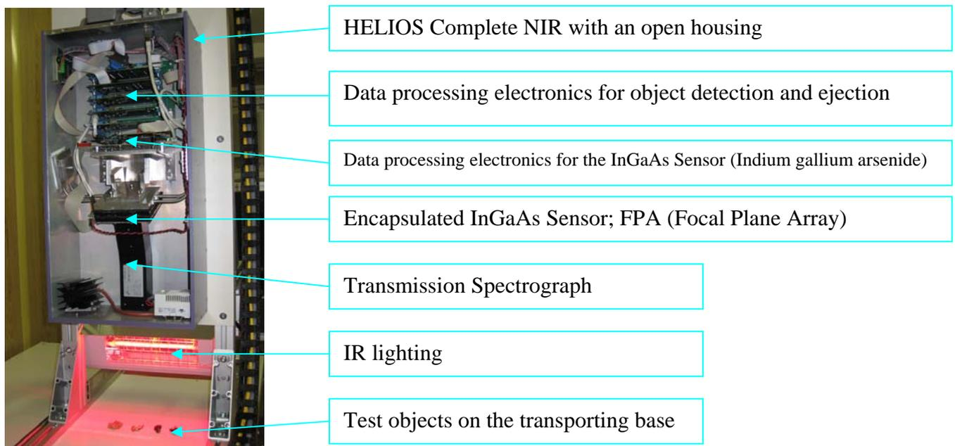
*Fig. 2: Test configuration, which consists of a swivelling arrangement of a transporting base, IR lighting and HELIOS Complete*
