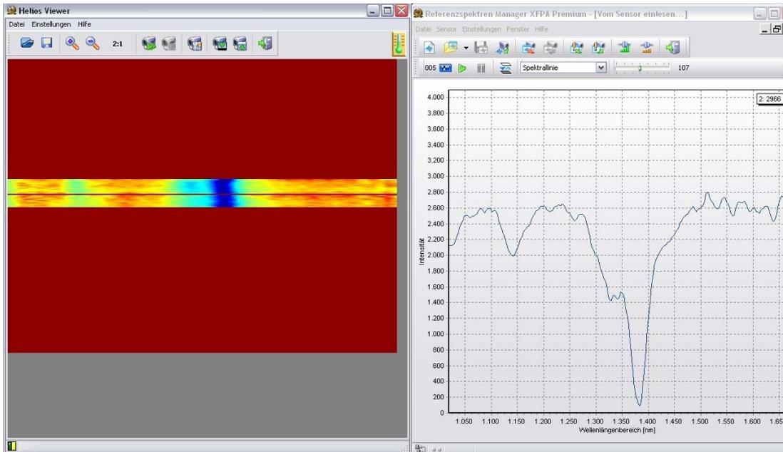
*Fig. 8: Spectra (1<sup>st</sup> derivation) of a larva. Larvae can also be clearly distinguished from blueberries and thus ejected as impurity.*
