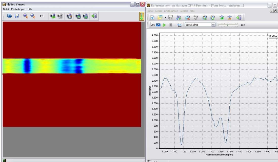
*Fig. 9: Spectra (1<sup>st</sup> derivation) of a worm. Worms can also be clearly distinguished from blueberries and thus ejected as impurity.*
