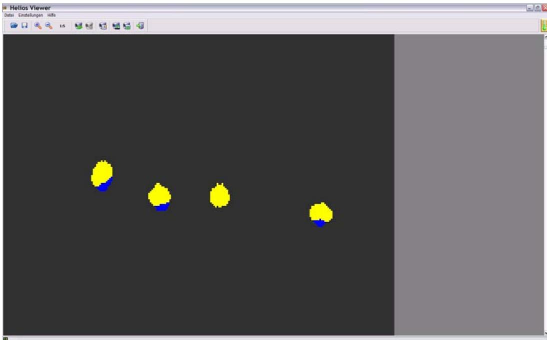
Fig. 7: Live recordings of blueberries with stems (blue), which are made by using **HELIOS Class**. Even though the stems are so small, they can be detected because the background does not generate any useful signal while the stem does.
