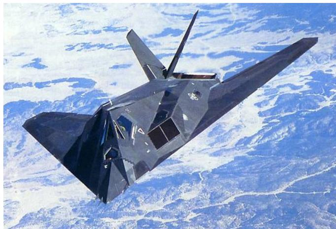
**Figure 5. Stealthy aircraft designed to avoid detection by active radar. The aircraft surface has a radar-absorbing material, and it's shape is designed to scatter any remaining radar radiation so that it is not returned to the emitter.**
