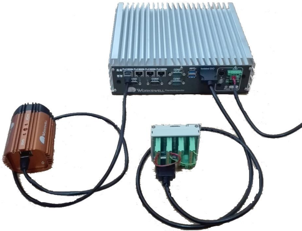
Wiring required cables to Central Passive Controller
