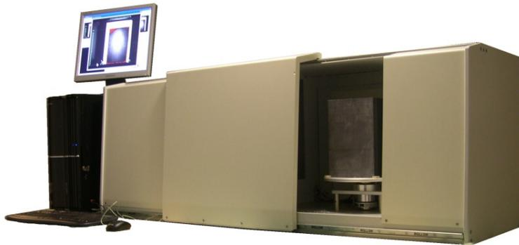
Fig. 1: System for Si ingot inspection, before cutting into wafers, based on an XS InGaAs camera.
