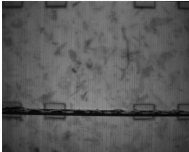
Fig. 2: Electroluminescence image of a Si solar under forward bias; image taken with a XEVA 1.7 320 TE1 camera.
