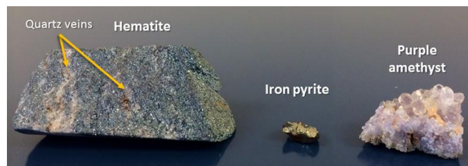
Figure 3 Visible image of a hematite drill core contaminated with quartz veins (left), iron pyrite (center) and amethyst (right).
