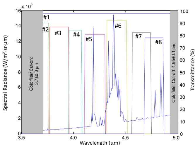
Figure 2 Blue (4.18 μm) and red (4.37 μm) spikes from the CO<sub>2</sub> overlaid on the transmittance of the 8 spectral filters for better evaluation.
